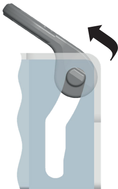
Pic. 16: Pivot the OPTILASH lashing ring into its usage position
