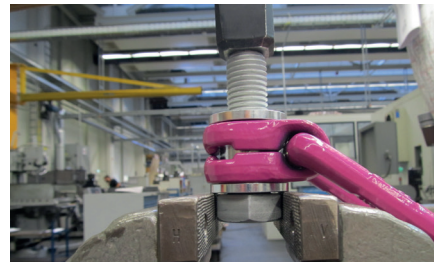
Pic. 7: Dismantling position of the VLBG-PLUS
